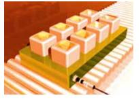
After filling resin, a palette carries workpieces into the hardening chamber automatically without stopping to change a palette.
