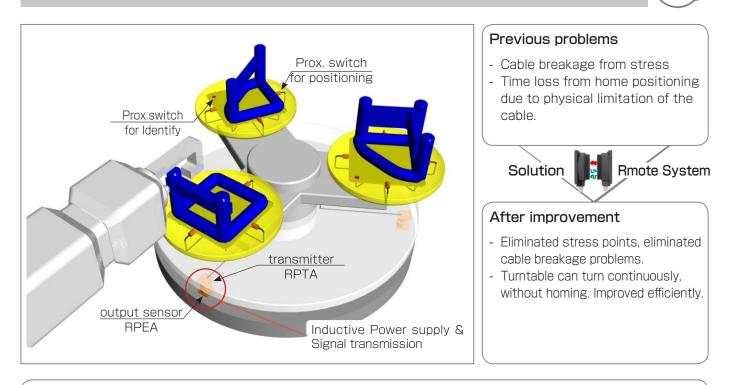
ApplicationContinuous cycle of Loading, welding and unloading. By using 3 jigs mounted on a turntable<br/>turning 120 degree at a time.<br/>Remote system supplies power to 8 proximity switches and transmits their switching state.
