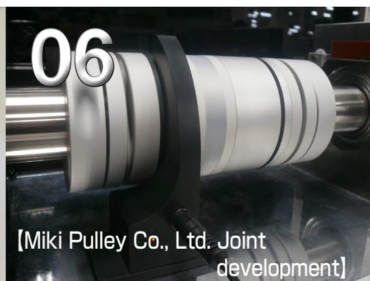
06 Ring coil + "C" shaped coil power supply to torque sensor
