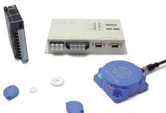
Writing a variety of information in the ID tag attached to the "object", and ID antenna, installed at any location, reads and writes its information. ID system to integrate the "information" and "object" is the key technology that can accommodate from automated mass production system to a flexible high-mix low-volume production system.
