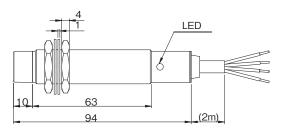
2 compensating lead wires Outer diameter : 3.2x5.1mm color of outer sheath : Blue, VX-G:7/0.3x2
