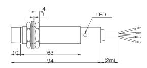
$\label{eq:compensating} \begin{tabular}{ll} 2 compensating lead wires & Outer diameter: $3.2x5.1mm \\ color of outer sheath: Yellow, JX-G:7/0.3x2 \\ \end{tabular}$
