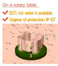
RS08 keeps transmitting power and detected signal while the table is rotating in a heated air or in showering of hot water.
